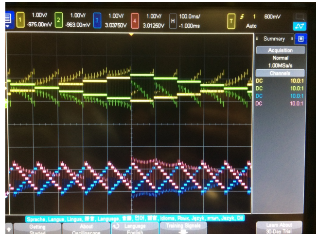
Figure 2: Sorted 2 elements using analog computer chip.
