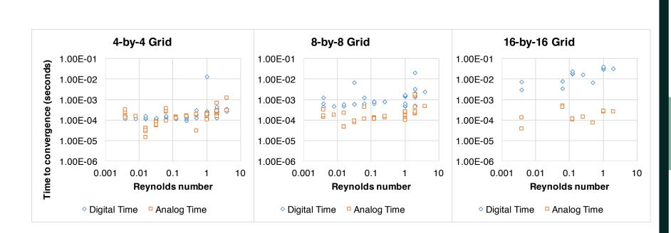
Analog approximate solutions for nonlinear equations are initial guesses for digital, which proceeds to high precision solution
