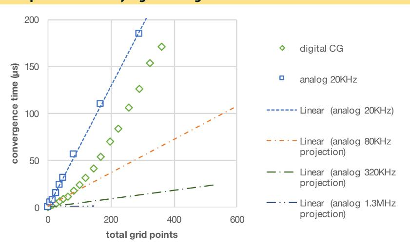
Analog linear algebra subroutine accelerates Newton's method, useful for finite difference solution of nonlinear PDEs
