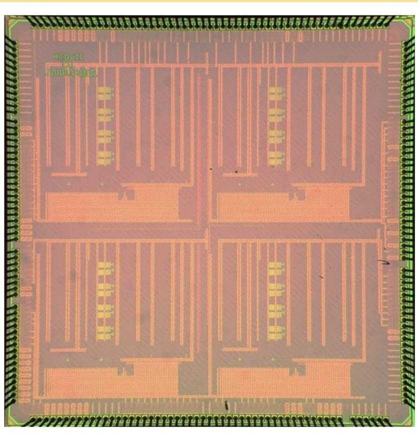
1.2V 65nm TSMC manufacturing process
