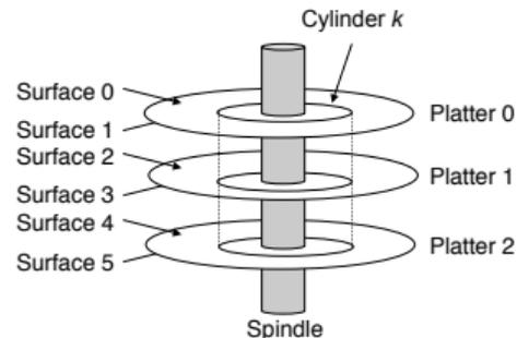
Figure: HDD. Image credit CS:APP
